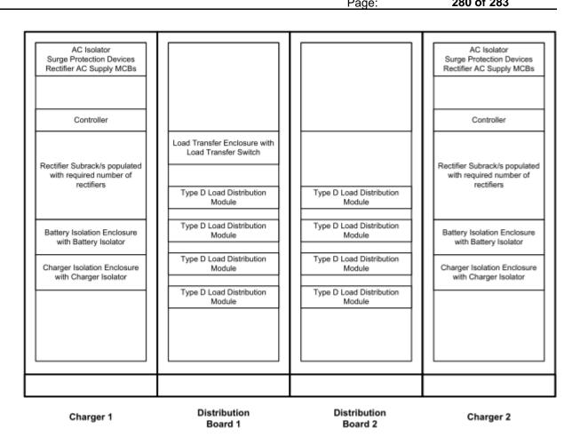
Figure H.12: 110V/220V Dual Battery Charger and Dual DC Distribution Boards Layout
