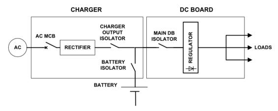
Figure H.2: 50/110/220V Single Battery Charger and DC Distribution Board Single Line Diagram
